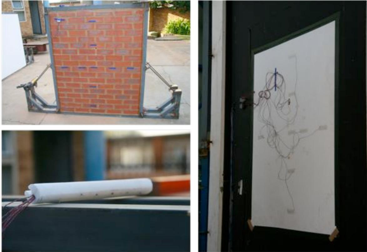
FIGURE 4: A typical specimen instrumented on the climate side in the steel construction jig before testing (top left), the XPS instrumentation probe used for measuring temperatures at various depths to establish thermal stability (bottom left), and a view of the climate side of an instrumented specimen mounted in the RGHB prior to testing (right).
